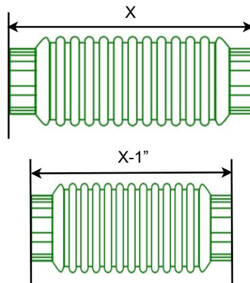
SPRING FORCE is the amount of weight or force it takes to compress a bellows 1".
