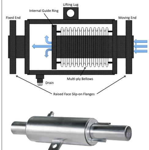
Keflex Externally Pressurized Expansion Joints
